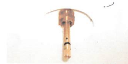
Step #7 Take the measured distance and add 3/8". This will give the amount to cut off the valve stem.
