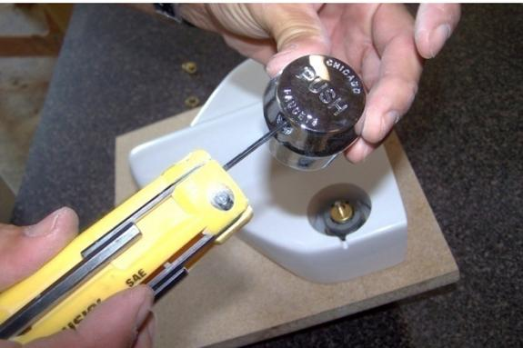
9. Loosen the set screw on the handle and slide it over the valve assembly. Push down on the handle cover before tightening the set screw
